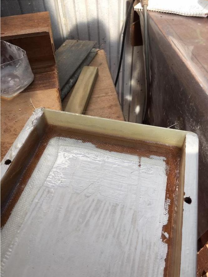
*The end then remade with a thin (3mm) but strong plate of epoxy and glass formed up on a broken piece of window pane, then glassed into the body of the tray.*
